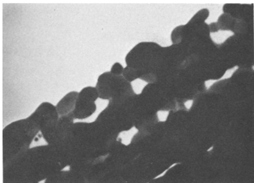
Figure 11 A TEM picture illustrating the grain structure within the filaments.
