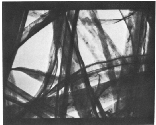
Figure 1 Extracted Nb filaments from a Cu–20 wt % Nb alloy after an area reduction of 7000.
